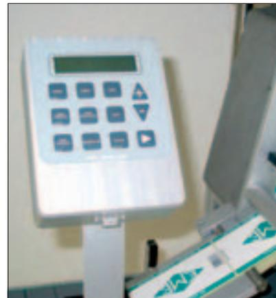
Optional separate keypad with display. It gives all the same control features as the built in keypad.
